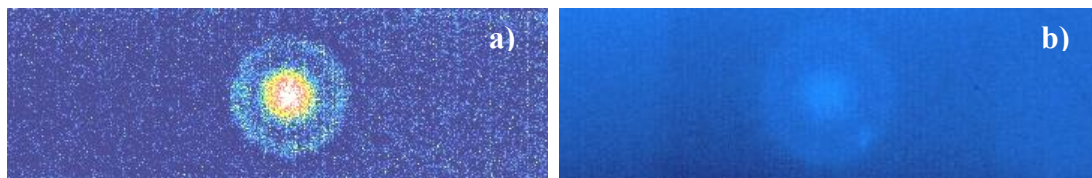
Fig. 10. LDR thermosonic imaging of FBH in PMMA plate at LDR frequency 7670 Hz: (a) - amplitude lock-in image (acoustic input \sim 200 \mu\text{W} ); (b) – temperature image at input power \sim 2 \text{ mW} .
