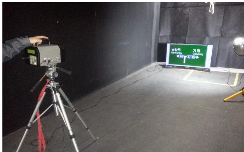
Figure 12. Luminance Measurement using the Dot Luminance Meter
