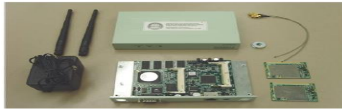
Fig 5: ARS hardware prototype, ARS software is then installed in Soekris wireless routers and evaluated extensively in our multi-radio WMN testbed.
