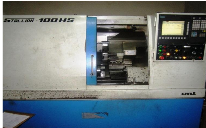
Figure 1: CNC Lathe machine (courtesy: R & D Centre for bicycle and sewing machine, Ludhiana)
