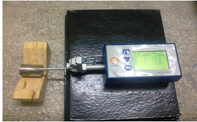
Figure 5: Surtronic 25 (Metrology lab, Mechanical department, SLIET)
