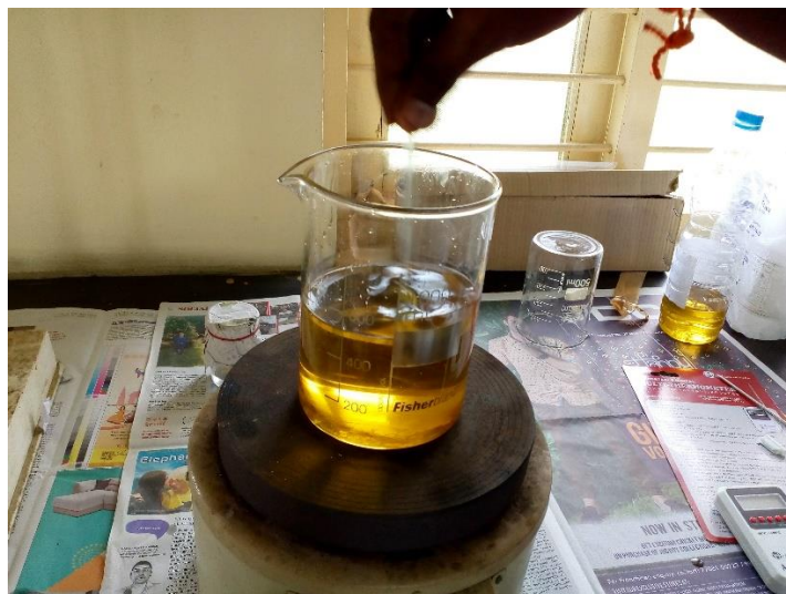
Figure 1: Heating of Crude Cottonseed Oil
