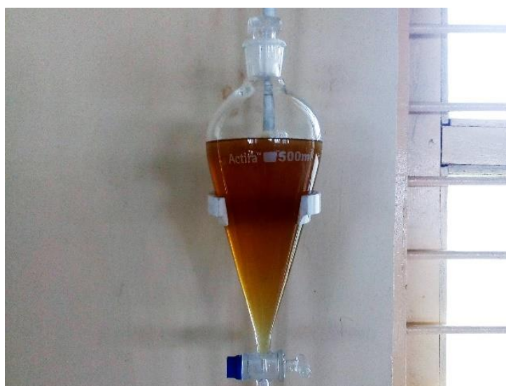
Figure 2: Heated oil with Sodium Ethoxide in the separating flask
