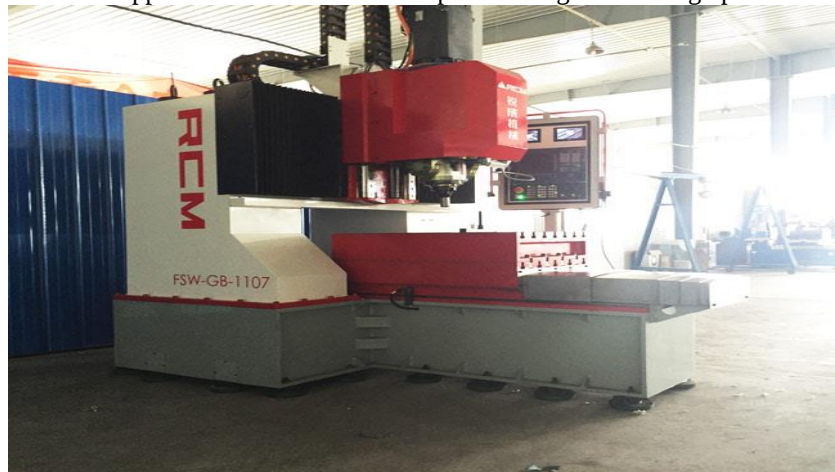
Fig.3. Experimental set up of FSW in BARC
