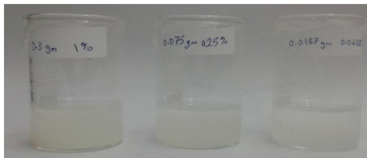
Fig. 5. Stability assessment of WO_3 /SDS nanofluids
