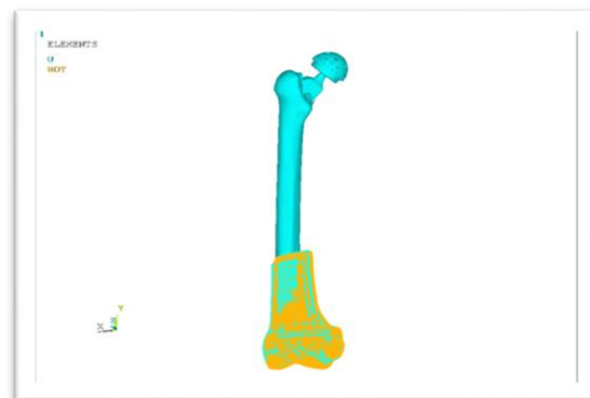
(b) Boundary condition (fixed in all DOF)
