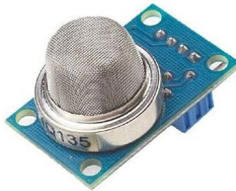
FIG 4: MQ-135 Alcohol Sensor
