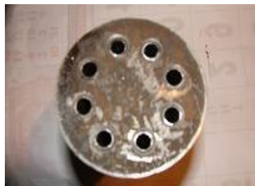
Fig. 1 C/S view of heat exchanger inner tubes.
