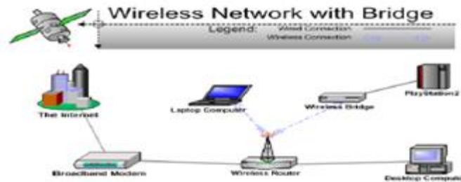
Fig.3 Wireless network with bridge
